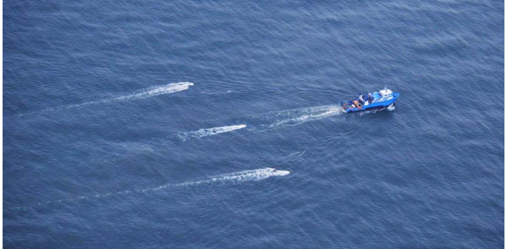
The R/V Brooks-McCall towing the P-Cable system in October 2013 in the Gulf of Mexico.
