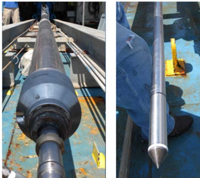
Figure 2. “CPT-Stinger” with a 11.6-m (38-ft) barrel equipped for short push
