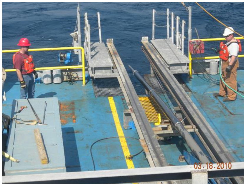
Figure 3. Deployment of the “CPT Stinger” from vessel stern
