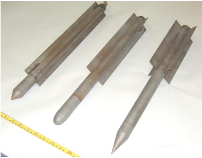
Figure 4: Model penetrators tested in Gulf of Mexico clays
