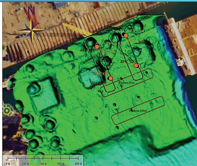
Figure 3. Plan view of Keppel AmFELS dock facility, channel bottom bathymetry, and core/CPT locations. Initial stacking location (black pontoons outlines) and revised location (red-outlined pontoons).
