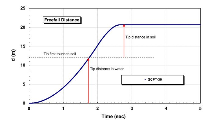
The program also calculates and logs the proper tip resistance baseline, friction sleeve baseline, pore pressure baseline. Now having a table of instantaneous velocity measurements coincident with the tip resistance, sleeve friction, and pore pressure measurements acquired 200 times per second, the program also individually adjusts the values of for tip resistance and sleeve friction to account for rate effects on these measurements.
