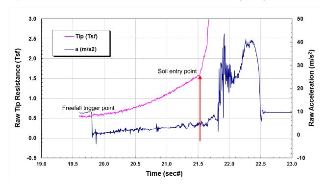
From these selected points, the program then integrates the acceleration values with respect to time from the freefall Trigger Point to the post-freefall At-Rest Point. This integration represents the velocity profile over time during this specific time interval. The derived instantaneous velocities are plotted below for the first 5 seconds after freefall trigger for this example from site gCPT-30.
