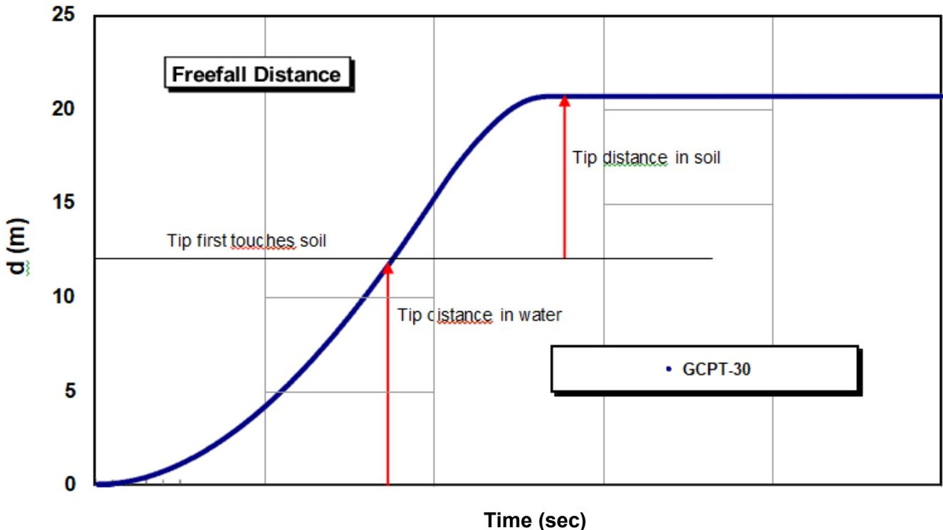
The program also calculates and logs the proper tip resistance baseline, friction sleeve baseline, pore pressure baseline. Now having a table of instantaneous velocity measurements coincident with the tip resistance, sleeve friction, and pore pressure measurements acquired 200 times per second, the program also individually adjusts the values of for tip resistance and sleeve friction to account for rate effects on these measurements.
