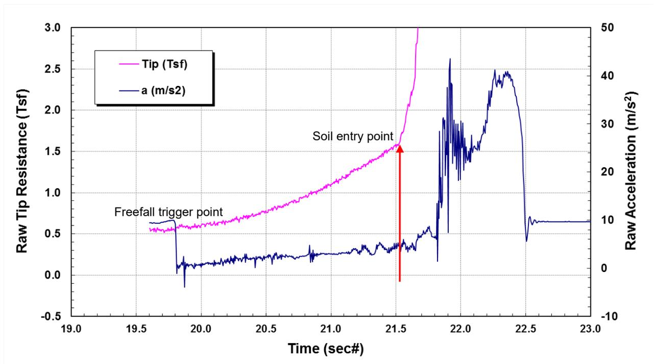
From these selected points, the program then integrates the acceleration values with respect to time from the freefall Trigger Point to the post-freefall At-Rest Point. This integration represents the velocity profile over time during this specific time interval. The derived instantaneous velocities are plotted below for the first 5 seconds after freefall trigger for this example from site gCPT-30.
