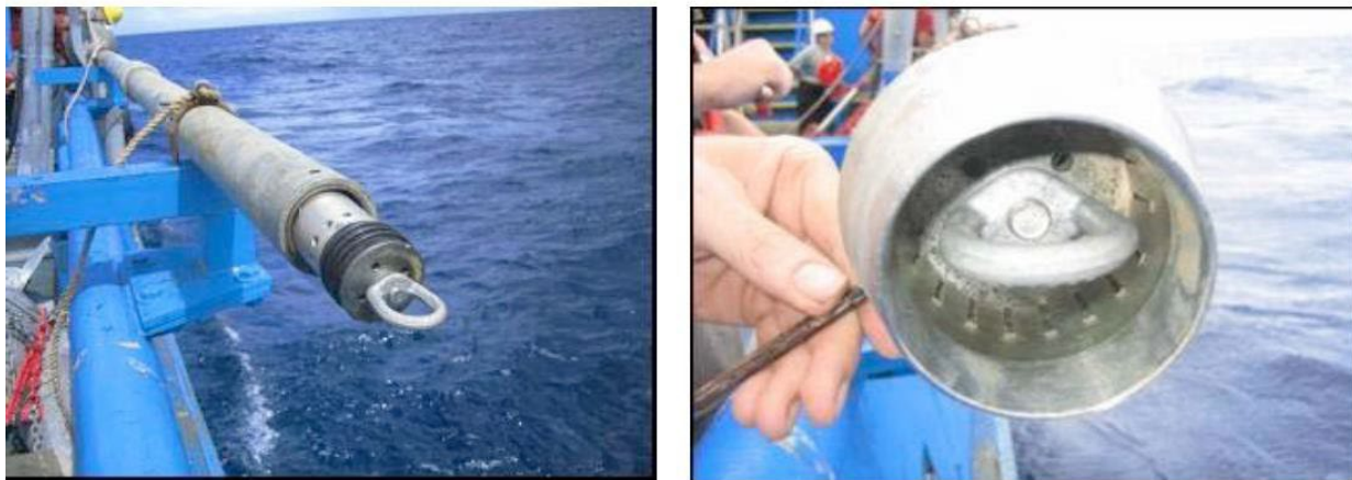
Figure 5) Barrel End Of The PC Rig With Piston Showing
