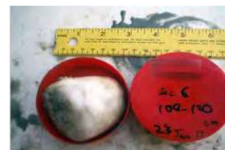
Gas hydrate fragment from oil stained core
