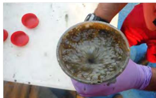
Core outgassing due to presence of gas hydrates
