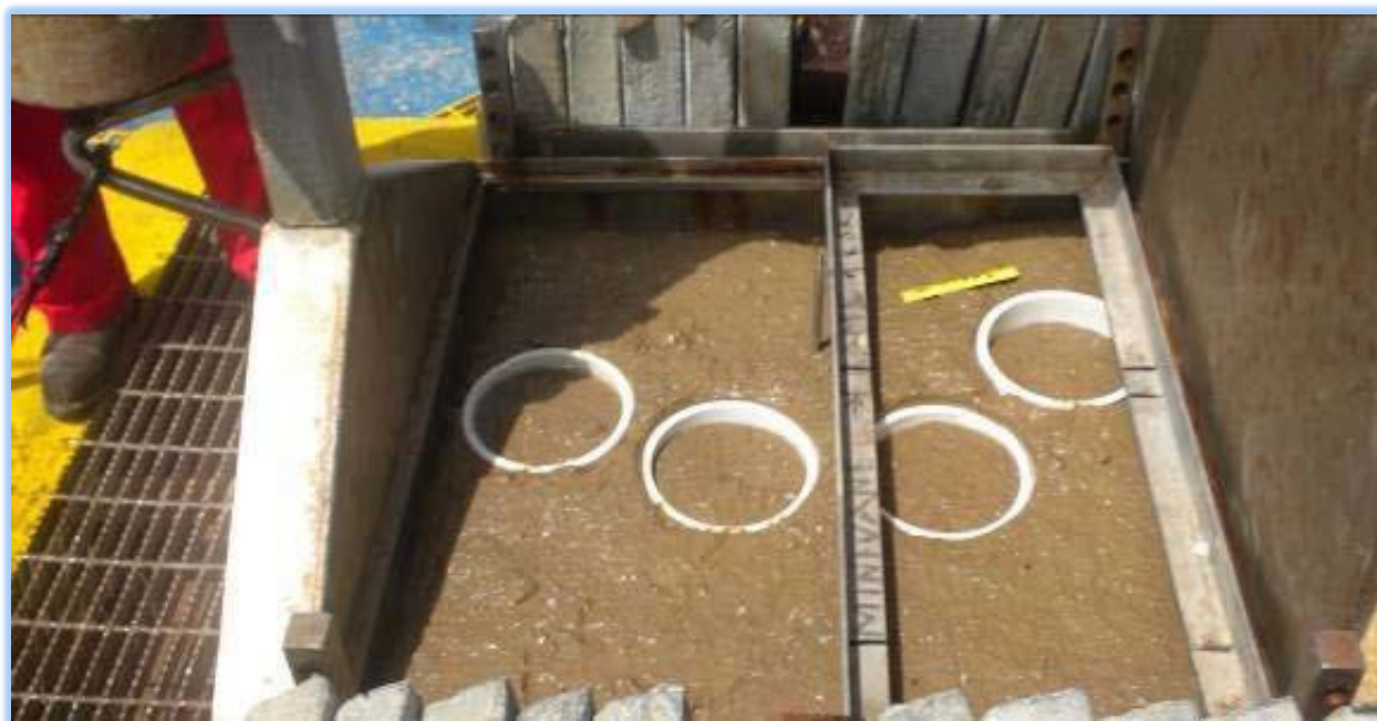
Figure 7) Box Core Sub-Sampled With Push-Core Tubes
