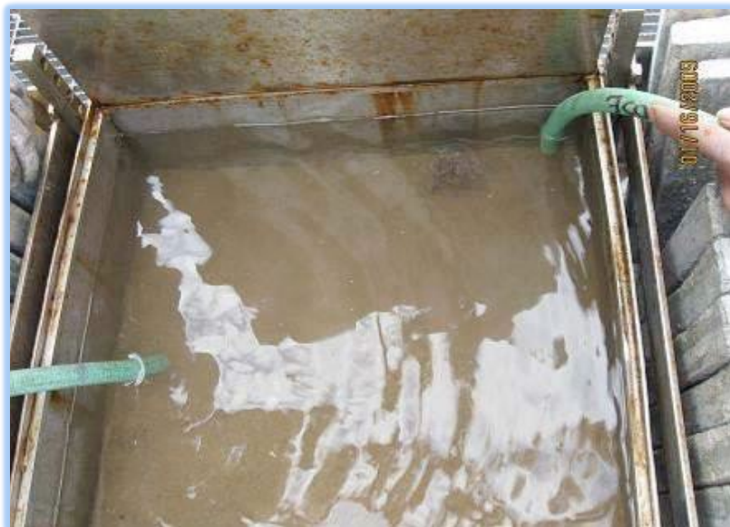
Figure 3) Siphoning Water From The Top Of A Box Core Sample
