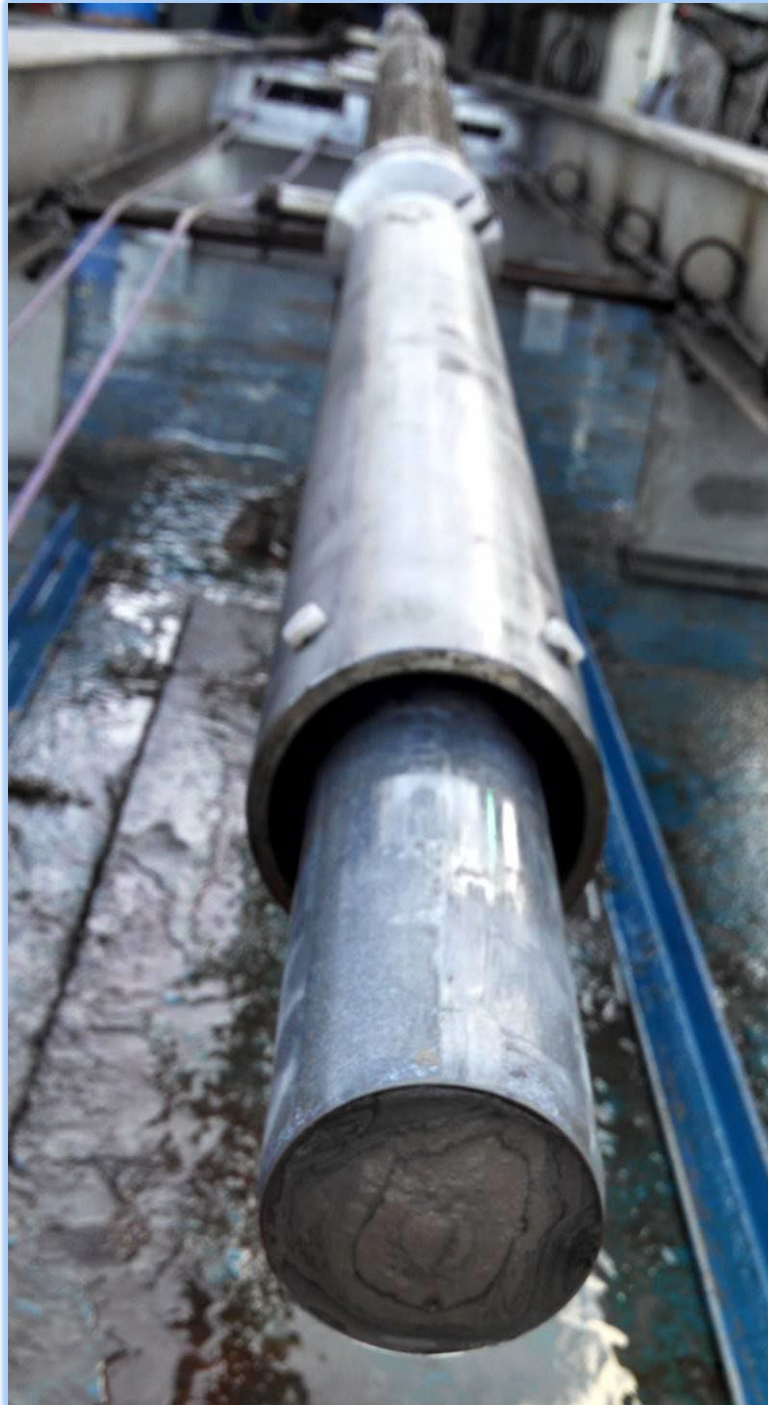
Figure 3) Photo Of The Stinger Sampler Shelby Tube With A Soil Sample From 40 M Depth
