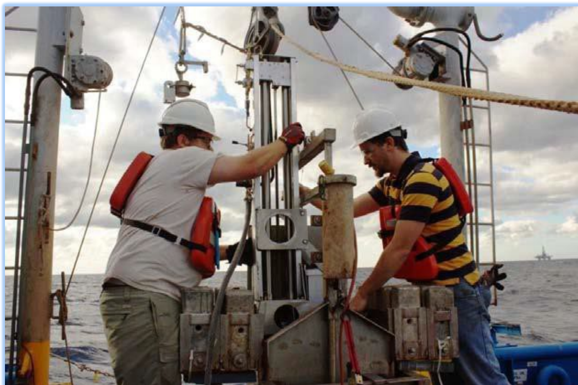
Figure 6) T-Bar Measurements On Box Core
