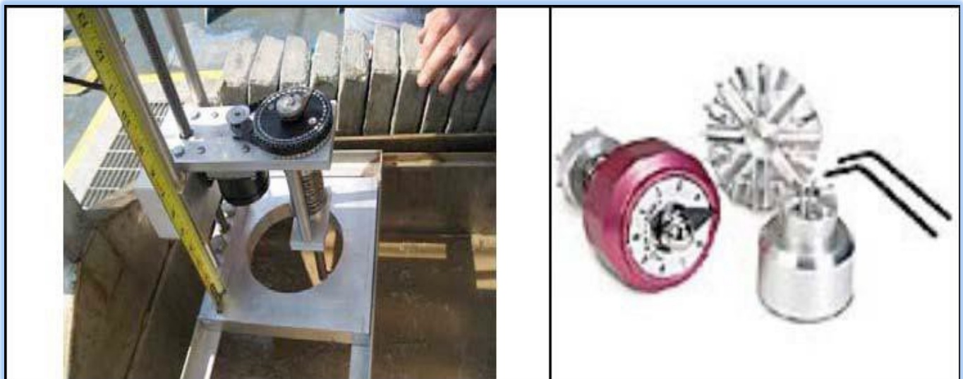
Figure 5) Miniature Vane On Box Core And Torvane
