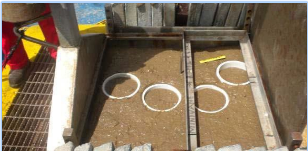
Figure 6) Box Core Sub-Sampled With Push-Core Tubes
