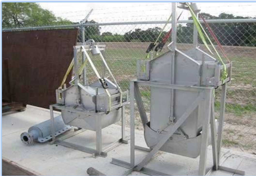
Figure 1) TDI-Brooks Half-Meter And One-Meter-Deep Box Coring Rigs
