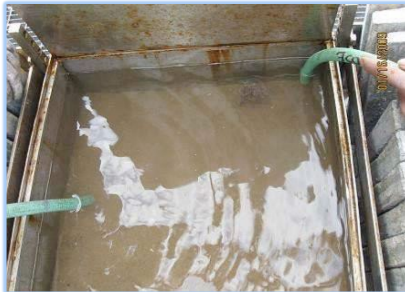
Figure 2) Siphoning Water From The Top Of A Box Core Sample
