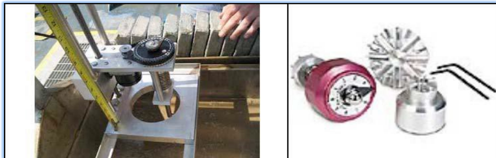
Figure 4) Miniature Vane On Box Core And Torvane
