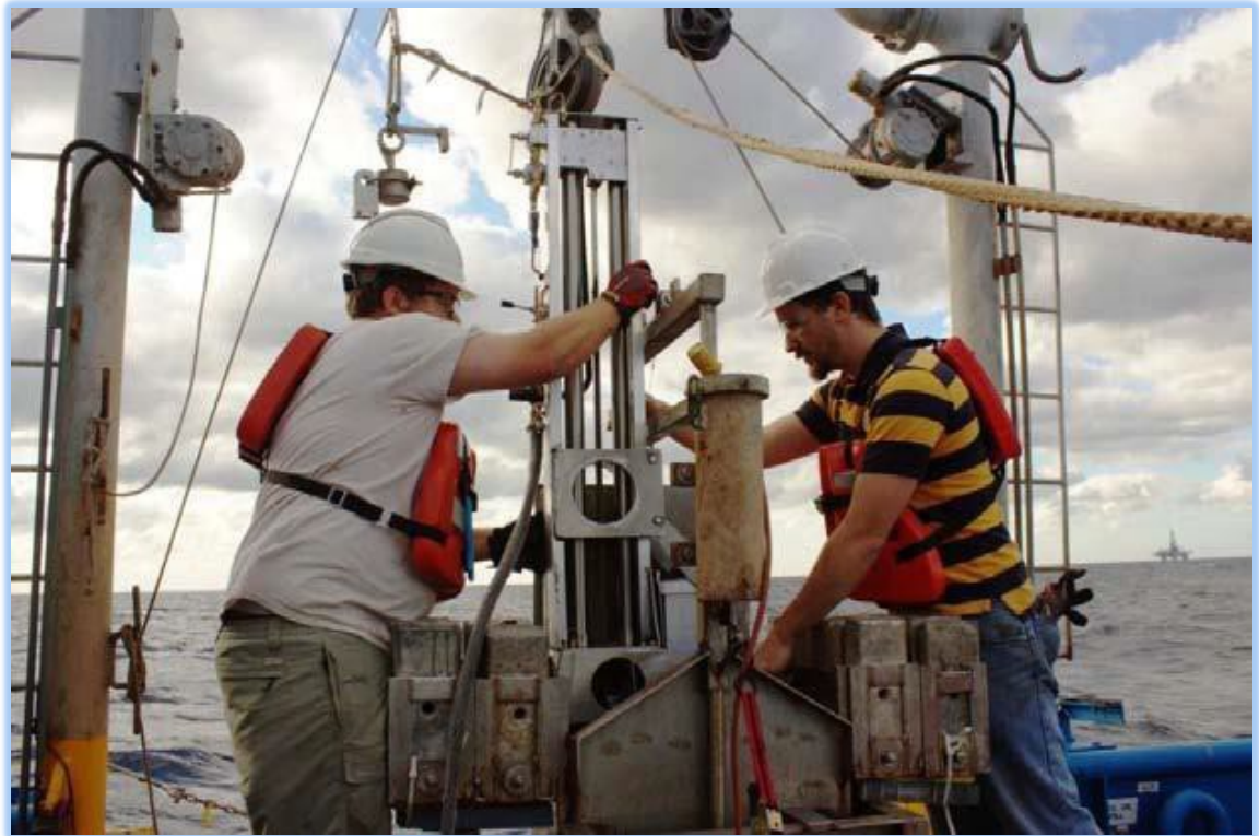
Figure 5) T-Bar Measurements On Box Core
