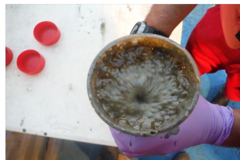
Core outgassing due to presence of gas hydrates
